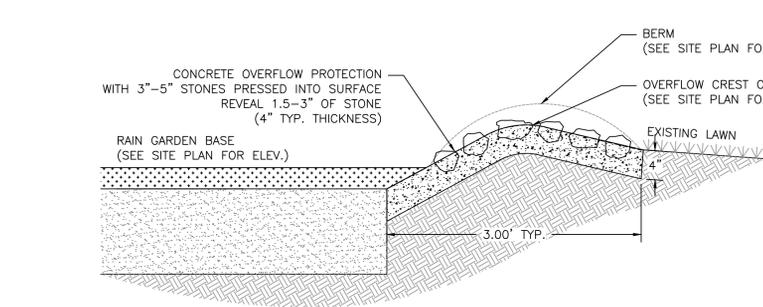
4 OVERFLOW PROTECTION CROSS-SECTION
