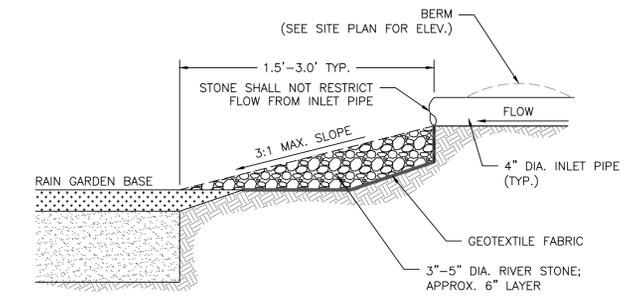
3 INLET PROTECTION CROSS-SECTION
